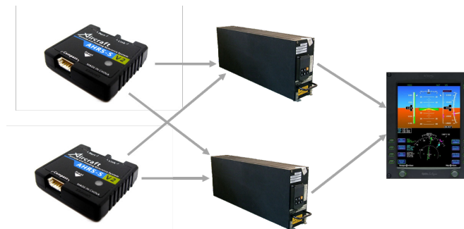
Figure 10: Basic architecture involving redundancy
